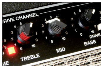
Three-band rotary EQ
