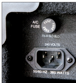
Easily replaceable fuse on a bass amp
